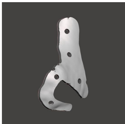
Fig 7: Final PSI Plate Design with Screw Holes in Meshmixer.
